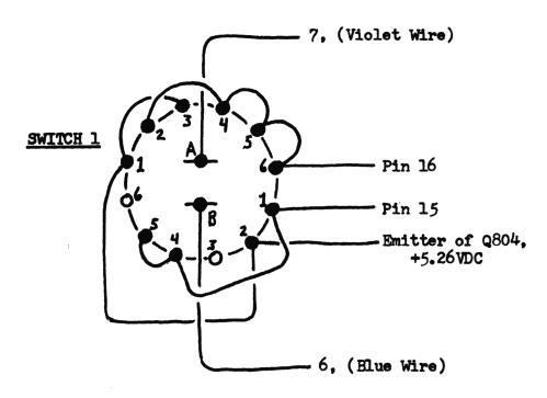
6. Wire-up a SPST switch as below and install per locations marked:
