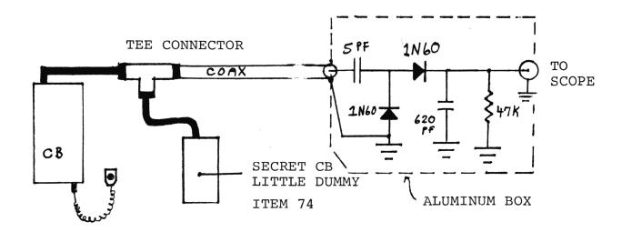
The above detector was built into a small aluminum mini box with an S0239 on one end and a cable to the scope on the other end. Here is how to use this detector with your scope.
