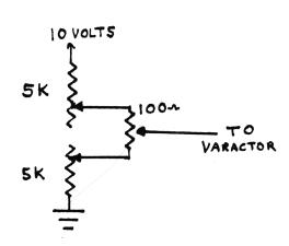
5K Pot is a Dual Pot. Resolution of above circuit is about 4 times better than a 10 Turn Pot! (If you can live with that many adjustments.)
