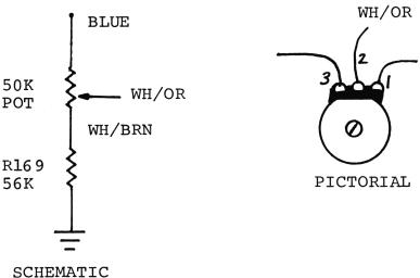
We are going to wire the RF gain so that the receiver is always on maximum sensitivity. This is accomplished by wiring like this:
