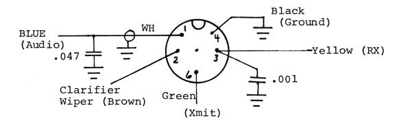
Unsolder all wires and then remove the jack. If you are not sure you will remember, label wires (such as, Black #4) before removing. Install a new 4 pin jack and wire up as shown below:
