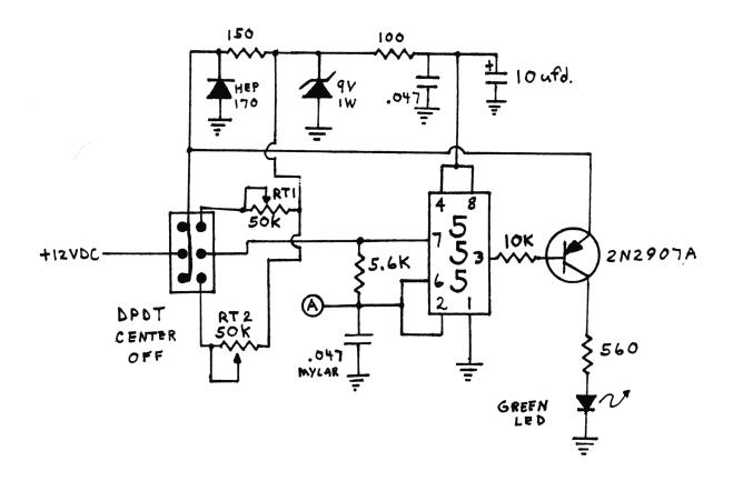
Adjust RT1 so output frequency is 879 hertz (28 MPH).
