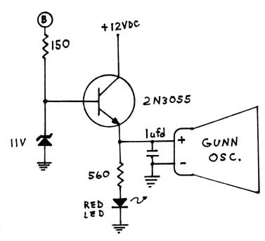
Add a lufd/25VDC capacitor on Gunn Oscillator for harmonic suppression.
