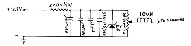
This circuit effectively isolates the reference voltage from all other circuits that could cause voltage fluctuation to the VCO.
