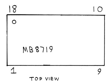
On the MB8719 Chips, for some reason, Pin 1 is not where the dot is, that is Pin 18. So be careful when you locate Pin 10.
