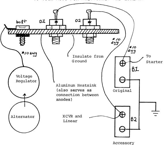
D1 and D2 act as one way switches. The action of these two is that of isolating the independent batteries from both discharging. Select high current common ANODE type stud rectifiers—such as those available from Poly-Paks(150 amps, 25PIV).
