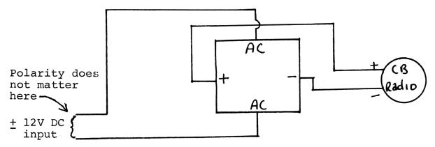
Bridge Rectifier - 25amp, 25 PRV Mount inside chassis.
