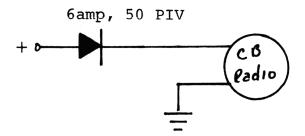
If connected up backwards, nothing will happen due to reverse bias which causes blocking action of diode. When connected properly, diode conducts, and radio will be ON.
