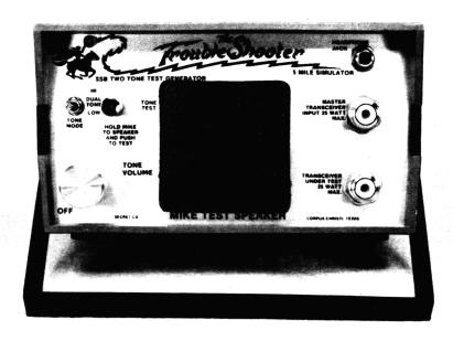
UNIT FEATURES A 5 MILE SIMULATOR FOR TRANSMITTER/RECEIVER TESTS (20 MILE SIMULATOR HAS BEEN ELIMINATED FROM PRODUCTION MODEL DUE TO UNAVAILABILITY OF SPECIAL PARTS); DUAL TEST TONES FOR TUNE-UPS; HEADPHONE OUTPUT JACK FOR MODULATION AUDIO CHECKS; DUAL 25 WATT DUMMY LOADS; WORKS ON INTERNAL 9V BATTERY AND HAS A JACK FOR OPTIONAL AC ADAPTOR.
