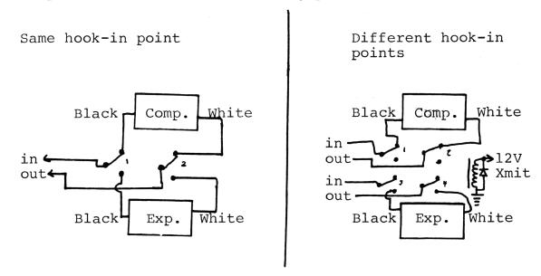
\*Relay is 4PDT Radio Shack #275-214 12VDC @ 75ma. or equiv.
