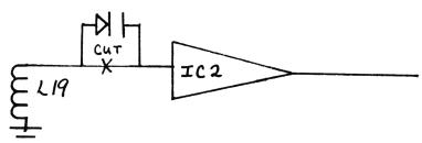
There is still some confusion concerning page 17 in Volume 8, and page 29 of Volume 9, concerning the Xtals. It was unfortunately omitted in Volume 8, that you must use an oscillator circuit in which the Xtals can oscillate and therefore feed that frequency into the location of the removed capacitor. In Volume 9, the schematic shown is NOT the oscillator circuit. The circuit outlined is simply for electronically switching
