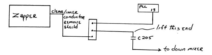
To get full coverage from 26.515 to 27.855 I replaced D201 Varactor with a Super Clarifier Diode (order our item #28), and adjusted L203.
