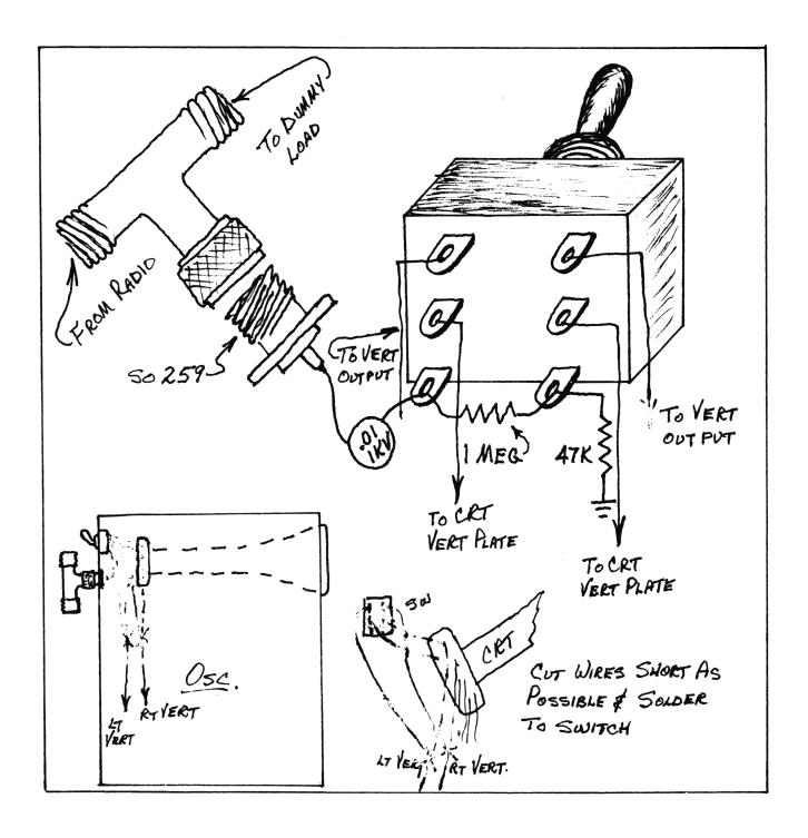
Install DPDT miniature toggle switch on back of oscilloscope and mount SO 259 as close as possible to switch and back of CRT so you do not have to extend the leads any more than necessary. The vert. cont's. will not be operational. Sync & Horizontal will need to be adjusted as necessary. To return to normal operation throw the switch.
