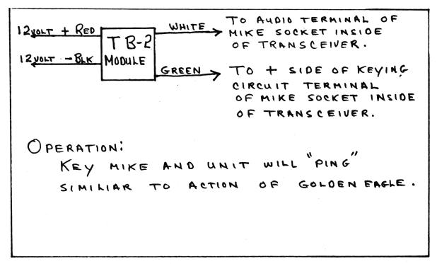
D&J Electronics, Inc. has brought back the ping because of the many requests for this popular unit. The simple installation of the unit allows a ping similar to the ping the Golden Eagle produced. A toggle switch in the power line to the module will allow the user to turn it off and on.
