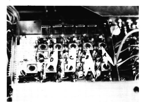
This photo shows the close-up view of pin #16 and the connection of the scope probe for the alignment of the coils.
