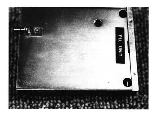
This photo shows the view of chassis where the PLL Unit and the counter unit were removed.
