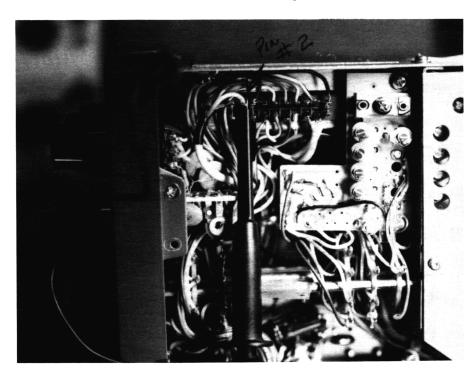
This photo shows the PLL Box that must be removed before the counter box may be removed.
