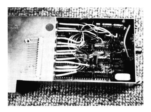
nside view of counter unit with the diodes installed.
