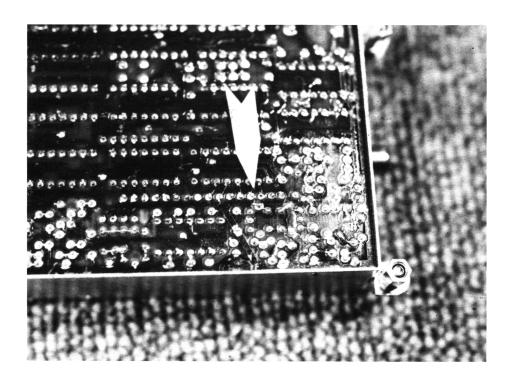
View of frequency counter board installed in radio. Modification completed, note short leads on diodes.
