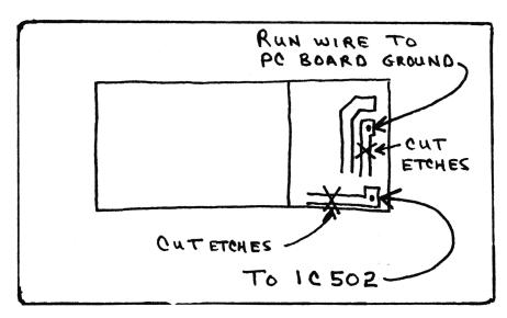
Replace D-702 with super diodes or equivalent for 6-8Kc slide. If more slide is necessary add a super slider diode in series with the newly installed maxi-tune. Be sure to lift anode end of maxi-tune and place in series from that side. The radio will now slide approximatley 11-15Kc.
