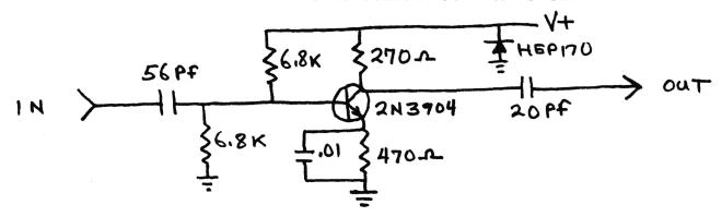
THIS UNIT MAY BE INSTALLED IN A RADIO. IT MAY BE USED AS A COUNTER PREAMP OR SCOPE AMP.
