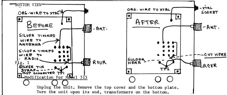
1. In the upper right corner, locate the small silver wire sticking up out of the board with nothing soldered to it. Cut the silver wire that goes from the receiver connector, indicated by an "X" (Fig. 1) and solder it to the silver wire sticking up out of the board.
