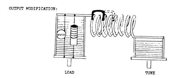
Factory Issue as depicted above. To modify, move strap on coil between "Load" and "Tune" from third turn (as per factory issue) to fifth turn (as indicated above).
