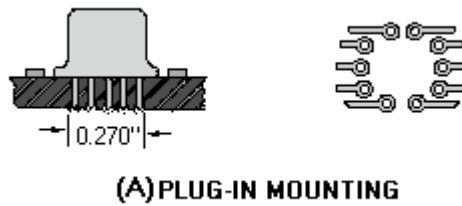
Figure 1-21A.—TO-5 mounting PLUG-IN MOUNTING
