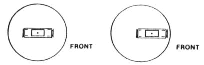
The best placement for maximum omni-directional performance is as close to the center of the vehicle as possible — on an automobile this will be the roof center. The center of the truck is also a good installation point.
