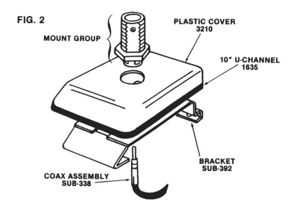
4. Insert end of coax through mount assembly from the bottom. Fig. 2.
