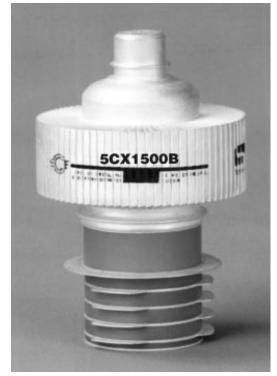
The Svetlana 5CX1500B is a high-performance ceramic/metal power pentode designed for use as a highly linear Class AB<sub>1</sub> linear amplifier. The pentode is ideal for VHF service and is recommended for use in FM broadcast transmitters. The 5CX1500B filament is precision fabricated in a cylindrical mesh configuration for exceptional mechanical stability and long life.
